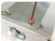
1、装回钢带压块，拧紧螺丝
