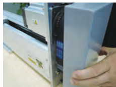
装回带轮罩并拧紧带轮罩四颗螺丝
