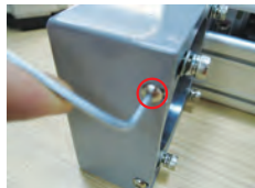
拧开带轮罩四颗螺丝并拆开带轮罩
