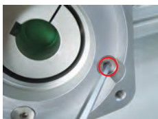
1、拆下电机座四颗螺丝
