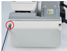
装回带轮罩并拧紧带轮罩四颗螺丝
