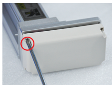
拧开带轮罩四颗螺丝并拆开带轮罩
