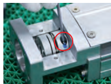
用内六角扳手紧固联轴器螺丝
