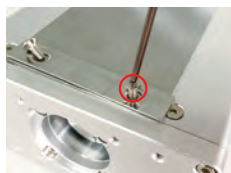
1、装回钢带压块，拧紧螺丝
