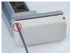
拧开带轮罩四颗螺丝并拆开带轮罩
