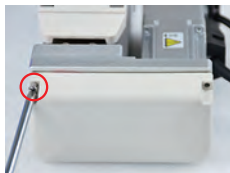
装回带轮罩并拧紧带轮罩四颗螺丝
