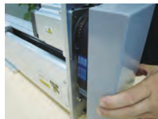
装回带轮罩并拧紧带轮罩四颗螺丝
