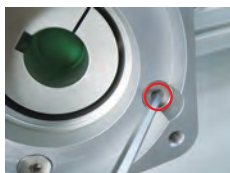
1、拆下电机座四颗螺丝
